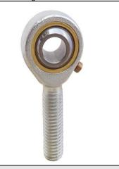
Ball: Gcr15 Steel, heat treated, HRC56 min; Precision ground,polished,hard chromium plated
